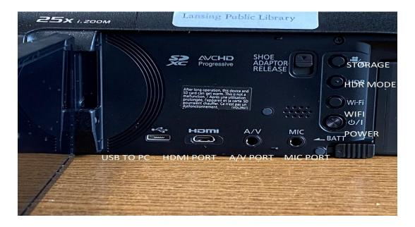
The Panasonic HC can be turned on by opening the flap on the side here and pressing the power button. The camera roughly has a 2-3 hour battery life, but this can vary depending on how much of the functions you use as well as how long it is running. It is recommended that when you are not using the Panasonic to turn it off to conserve battery life. This can be done by closing the flap, or pressing the power button in the same manner to turn it on.
