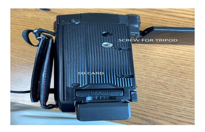
The bottom area holds the area where the SD card is installed in. You can take this SD card out by pushing up on it and then retrieving it from there. There is also the area of where you can screw in the Pansonic into the tripod that will out and available for use.
