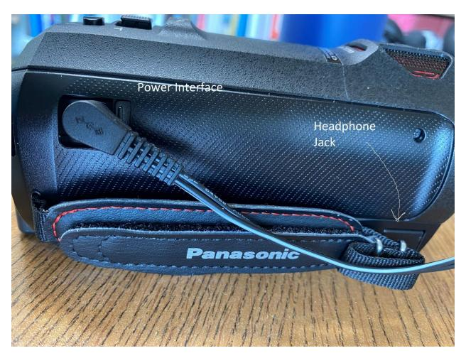
On the other side of where the main panel is, you will find the power input for the Panasonic. Plug the AC adapter into it to recharge the Panasonic. We ask that when you are done with your recordings, that you plug it into the socket. On the lower right hand corner, you will see an attachment to plug in a pair of headphones to the Panasonic...so you can better hear the volume as you record.
